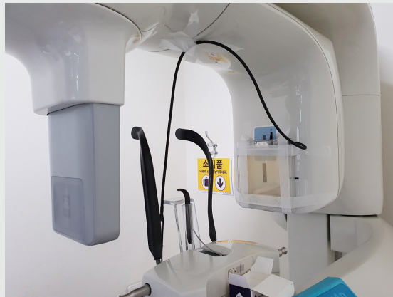
Figure. 2. The ionization chamber of DAP meter was positioned at the tube side of panoramic radiographic machine for the DAP measurement.
