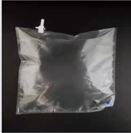
Figure 2. One isolated Pre-capsulated dental amalgam and 2 L of (4\pm 2)^\circ\text{C} Air in a Tedlar Bag
